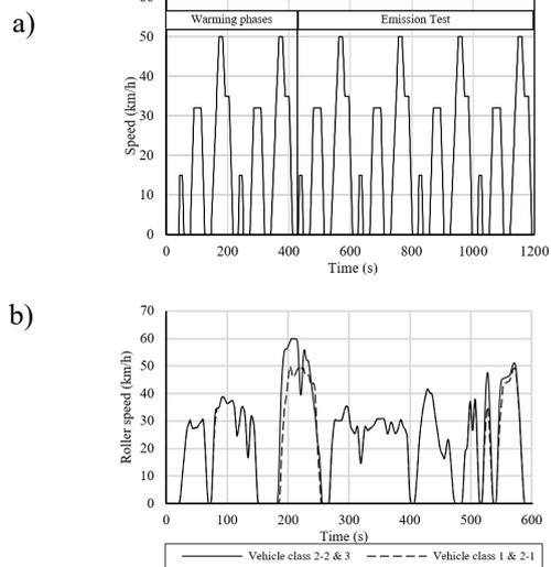
**Fig 3.** ECE R40 (a) and WMTC (b) driving cycles.
