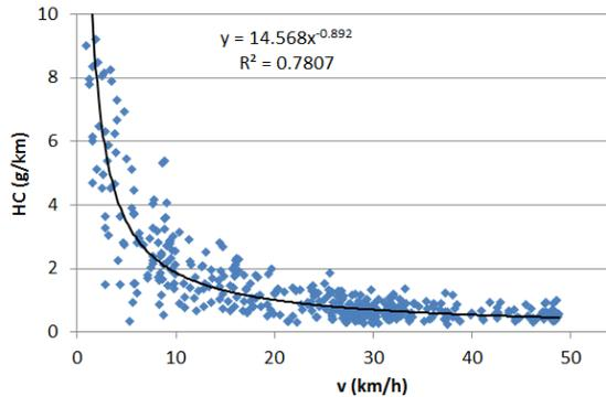
**Fig 4.** HC emission model, carbureted motorcycles with gasoline fuel.
