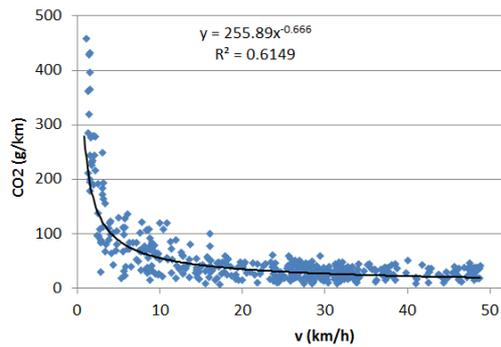
**Fig 7.** CO<sub>2</sub> emission model, carbureted motorcycles with gasoline fuel.
