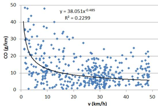
**Fig 5.** CO emission model, carbureted motorcycles with gasoline fuel.
