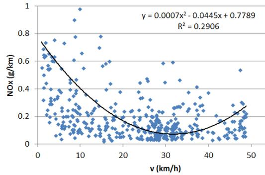
**Fig 6.** NO<sub>x</sub> emission model, carbureted motorcycles with gasoline fuel.
