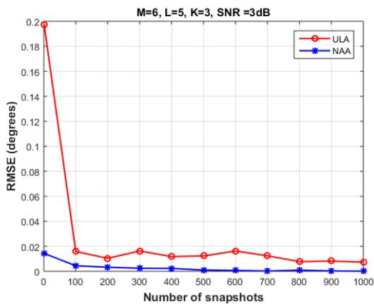
Fig.3. Accuracy comparison between ULA and NAA
