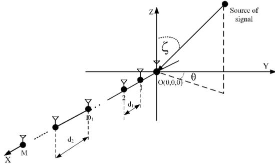
**Fig. 1.** Nested Antenna array in the coordinate system
