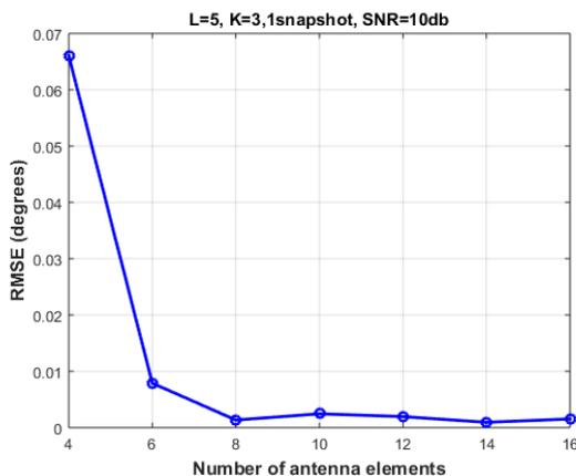
Fig.4. Impact of number of antenna element on accuracy of DOA estimation
