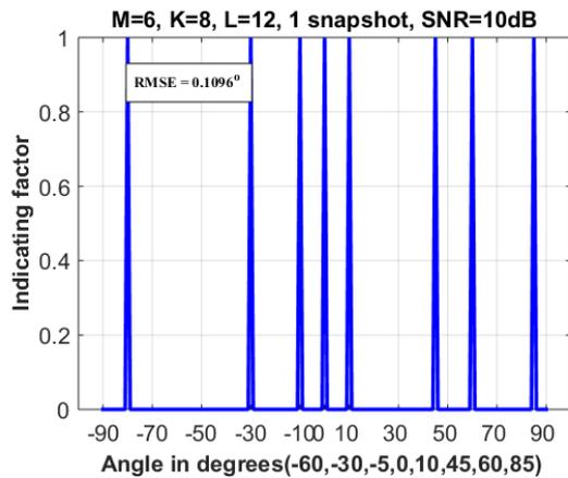
Fig.2. DOA estimation with NAA with one snapshot
