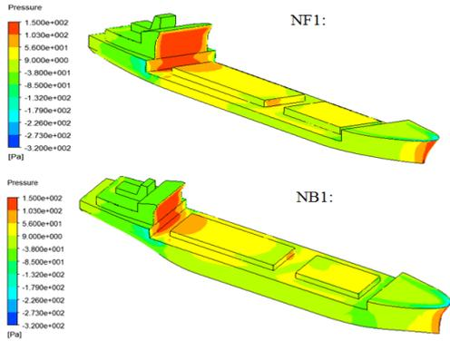
Fig. 8. Pressure distribution over hull surface of the ships, NF1 and NB1
