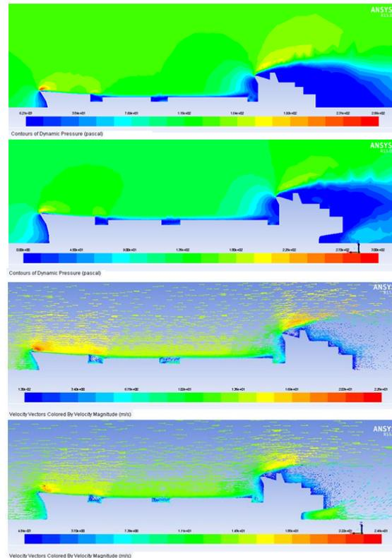
Fig. 7. Dynamic pressure distribution and velocity flow around hull at center plane of computed fluid domain of the ships, NF1, NB1
