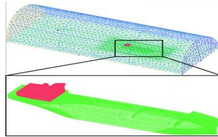
Fig. 3. Computed fluid domain and meshing
