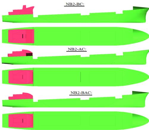
Fig. 12. New hull form proposed for the conventional ship at ballast condition, NB2
