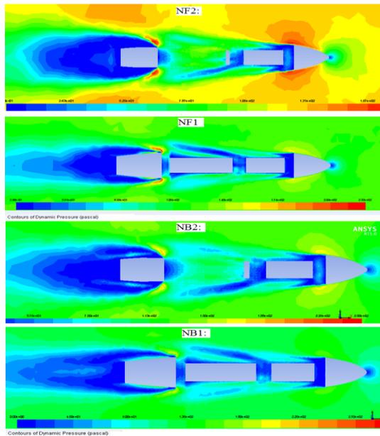
Fig. 9. Dynamic pressure distribution around hull at horizontal plane ( $z=0.18m$ ) of the computed fluid domain, NF1, NF2 and NB1, NB2
