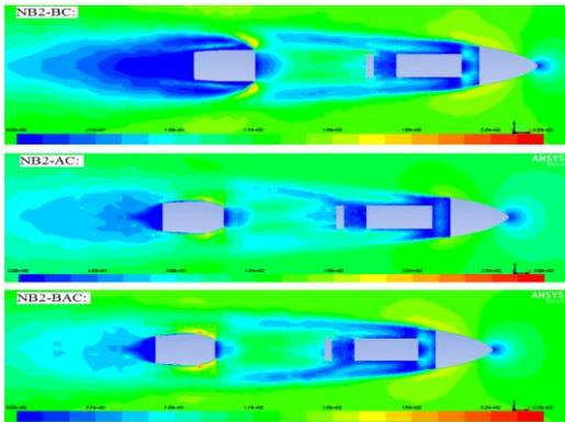
Fig. 18. Dynamic pressure distribution around hull at horizontal plane ( $z=0.18m$ ) of the new ships
