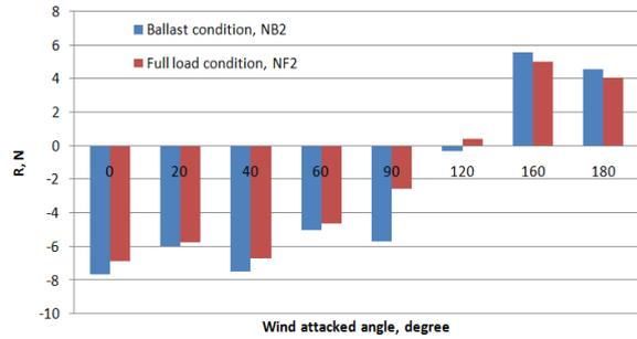
Fig. 5. Air resistance acting on the original ship at full load and ballast conditions
