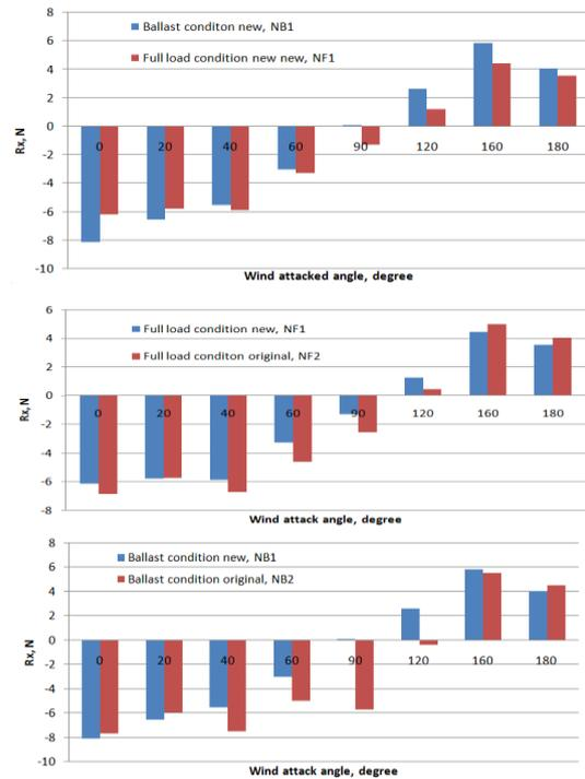
Fig. 10. Air resistance acting on the ships at full load and ballast conditions NB1, NB2 and NF1, NF2
