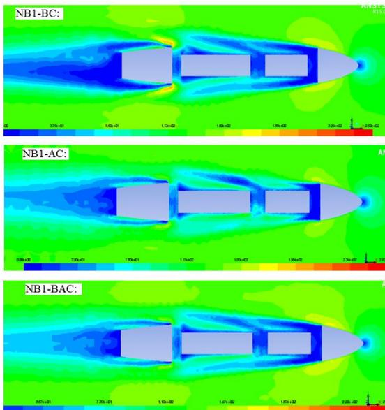
Fig. 14. Dynamic pressure distribution at horizontal plane ( $z=0.18m$ ) of the computed domain
