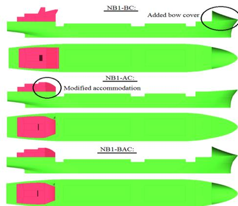
Fig. 11. New hull form proposed for the new concept ship at ballast condition, NB1
