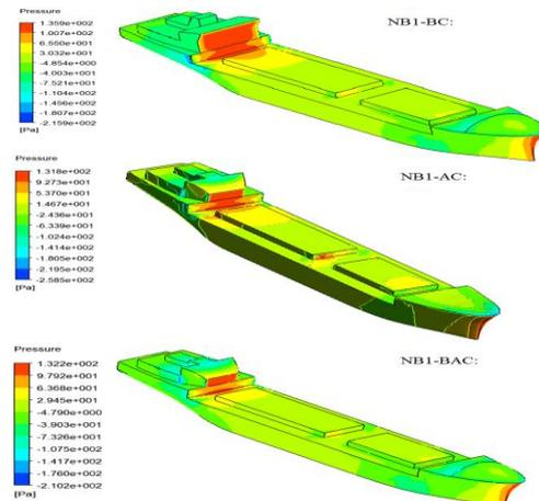
Fig. 15. Pressure distribution over hull surface of the new ships
