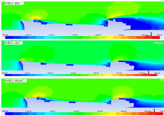
Fig. 17. Dynamic pressure distribution around hull of the new ships NB2 with AC, BC and BAC
