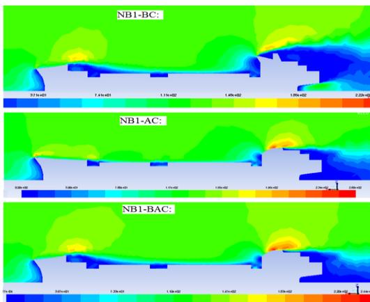
Fig. 13. New hull form proposed for the new concept ship at ballast condition, NB1
