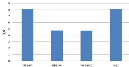
Fig. 16. Air resistances acting on the ships
