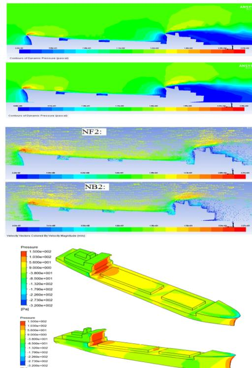
Fig. 4. Pressure and velocity distribution around hulls of the ships in full load and ballast conditions
