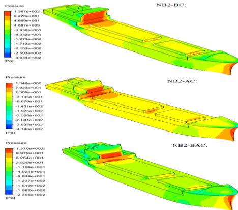
Fig. 19. Pressure distribution over hull surface of the new ships with AC, BC and BAC
