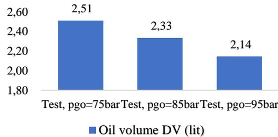
Fig. 8. The oil volume recovered in the proposed HRBS: experimental results under various pressure  $p_{go}$
