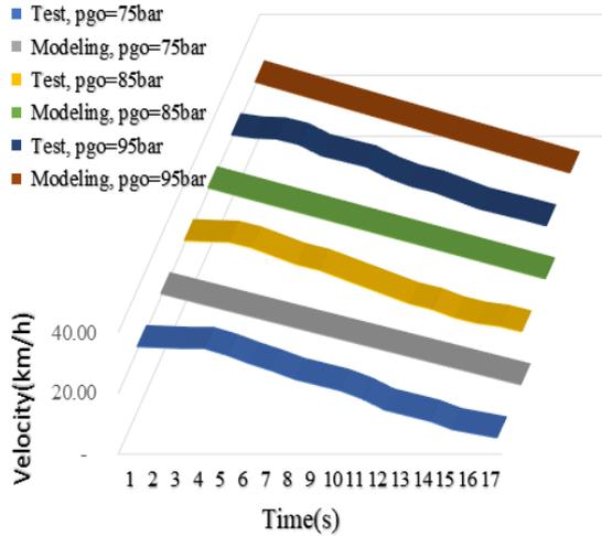
Fig. 6. Velocity versus time in the HRBS measured at various working pressures
