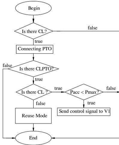
Fig. 2 The flow chart showing working of the proposed HRBS
