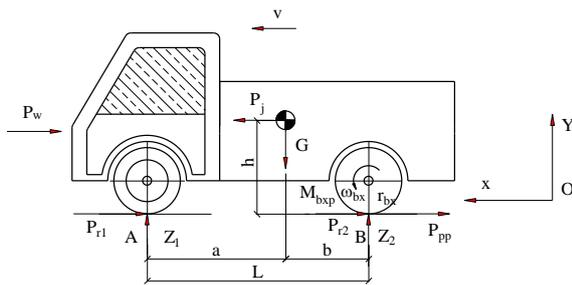
Fig. 3. Forces acting on the test vehicle
