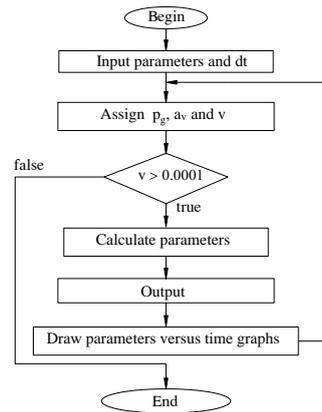
Fig. 5. The flow chart showing calculating steps in the proposed HRBS during the braking process
