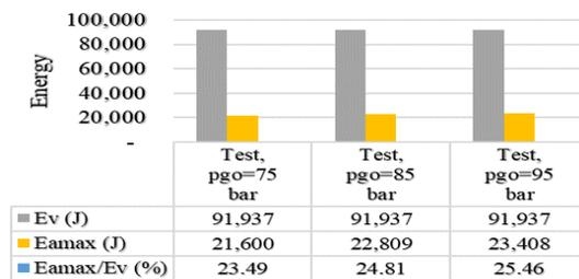
Fig. 9. Percentages of energy recovered in the proposed HRBS: experimental results under various pressure  $p_{go}$
