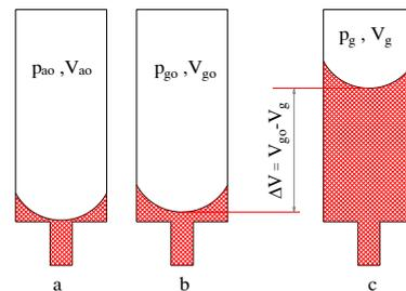
**Fig. 4.** The hydraulic accumulator and state of charge-SOC: a--The initial SOC, b- The low operating pressure and c - The high operating pressure
