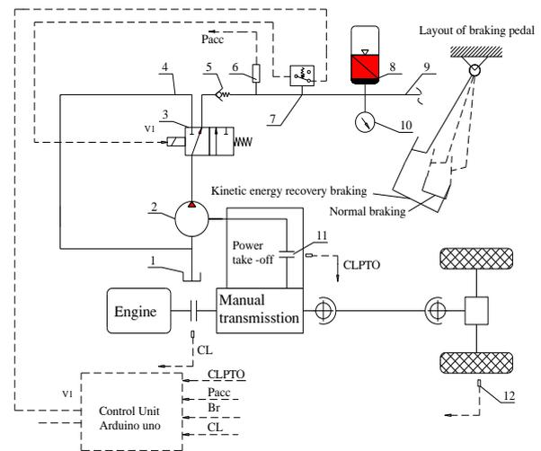
Fig. 1 The principle diagram of the proposed HRBS
