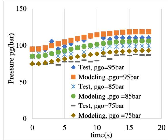
Fig. 7. Pressure versus braking time in the proposed HRBS: modelling and experimental results
