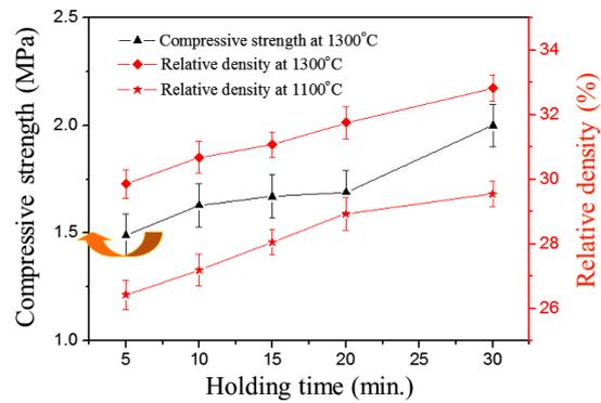
**Fig. 5.** Relative density and compressive strength of porous HAp scaffold depending on the holding time
