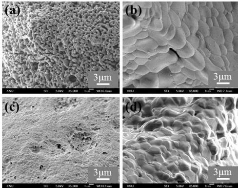
**Fig. 2.** SEM micrographs of pore frame of porous HAp scaffold depending on the sintering method, conventional sintering at (a) 1100°C and (b) 1300°C, microwave sintering at (c) 1100°C and (d) 1300°C
