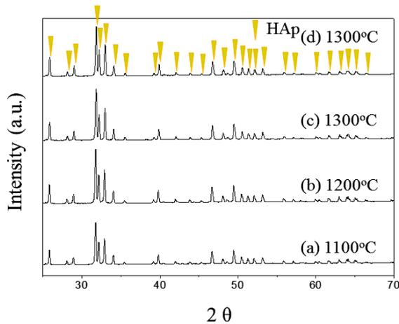
**Fig. 3.** XRD profiles of porous HAp scaffold sintered by (a, b, c) microwave sintering depending on the sintering temperature with 30 min of holding time and by (d) conventional sintering
