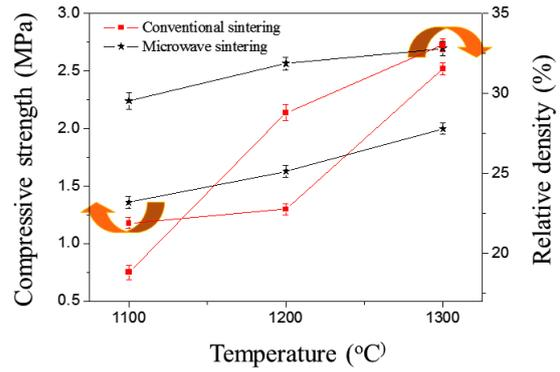
**Fig. 4.** Relative density and compressive strength of porous HAp scaffold depending on the sintering temperature and sintering method
