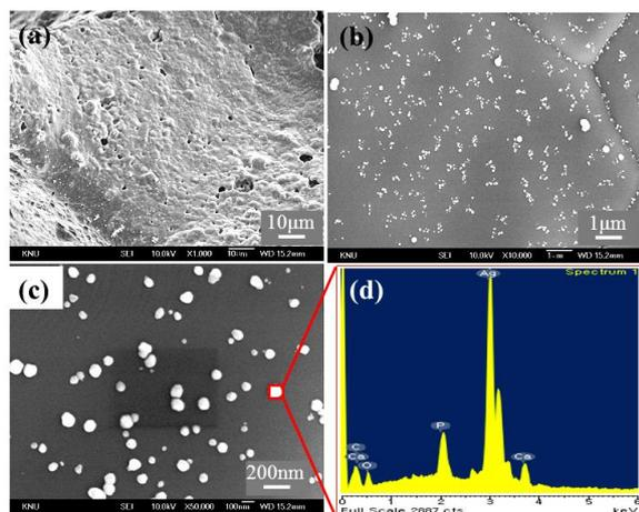
**Fig. 6.** SEM micrographs and EDS profile of nano-Ag coated porous HAp scaffold (a) pore frame, (b) enlarged image, (c) high magnification and (d) EDS profile
