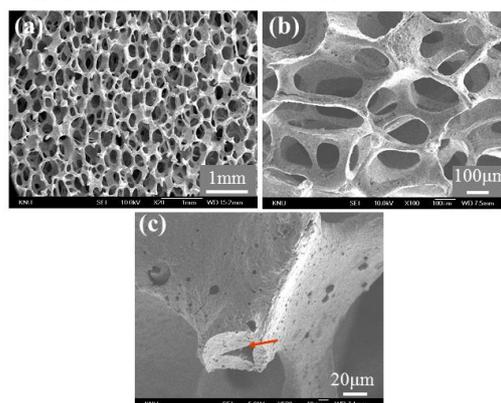
**Fig. 1.** SEM micrographs of porous HAp scaffold (a) low magnification, (b) enlarged image and (c) cross sectional view of pore frame
