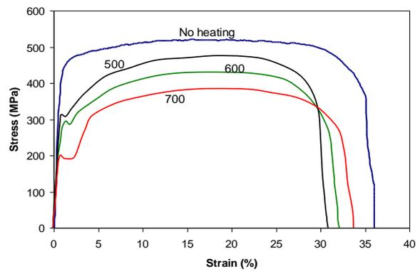
**Fig. 5** Stress – strain curves of the steels
