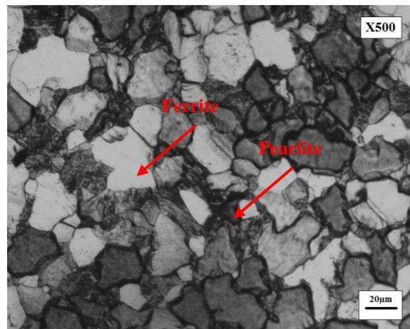
(b) Sample heated at 500  $^{\circ}\text{C}$
