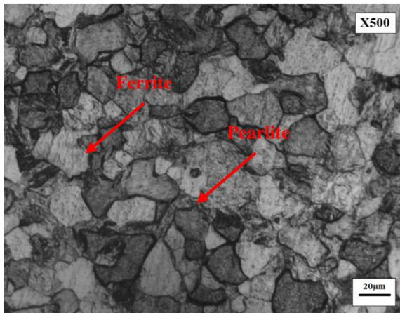
(c) Sample heated at 600  $^{\circ}\text{C}$
