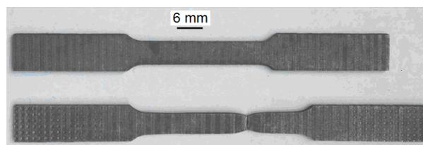
**Fig.1** The specimen for the tensile test
