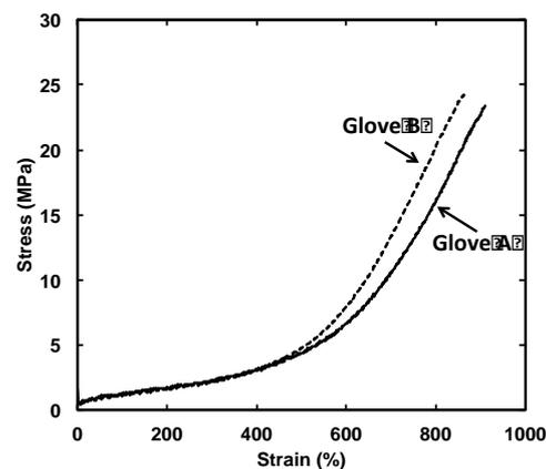
Fig. 3. Stress-strain curves of glove A and glove B
