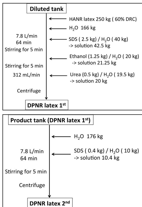
Fig. 1. Operation of Test plant
