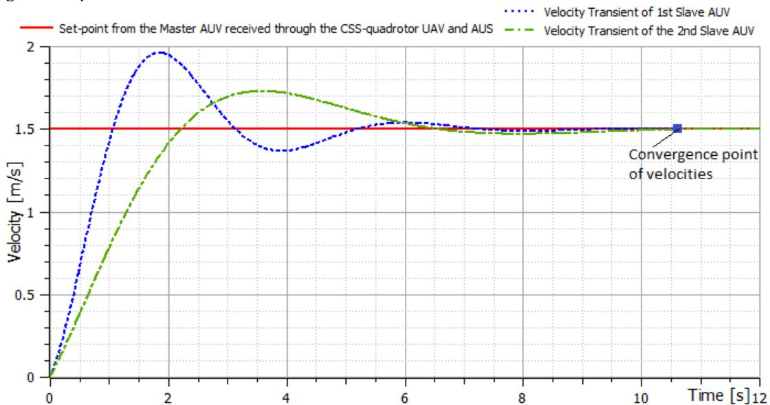
**Fig. 4.** Example of velocity convergence in a MAUVs flock.
