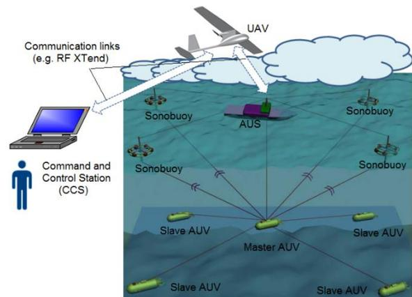
**Fig. 1.** Coordinated structure of a UAV and AUS/MAUVs team.
