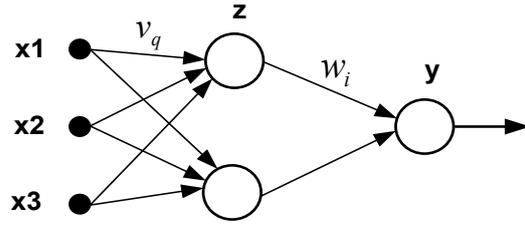
Fig. 2. Direct connection NN architecture [5].
