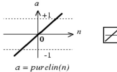
Fig. 5. The activation function  $a = \text{purelin}(n)$ .
