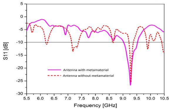
**Fig. 7.** The difference between impedance matching of antenna without metamaterial and with metamaterial
