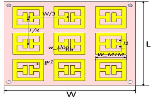
Fig. 5. MRS structure (a) structure and equivalent circuit of unit cell (b)
