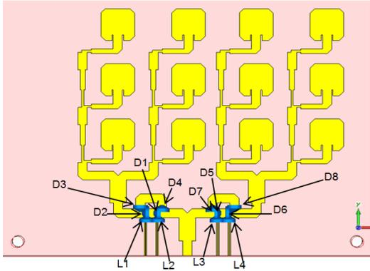
**Fig. 1.** The model of proposed antenna: top (a) and bottom (b)
