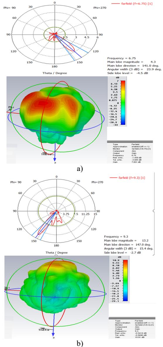
**Fig. 8.** The radiation pattern of antenna at center frequencies of 6.57 GHz (a) and 9.3 GHz (b)
