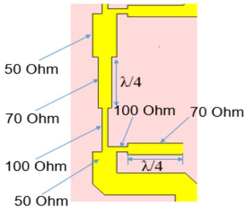
Fig. 4. The impedance matching for antenna
