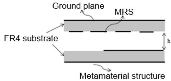
**Fig. 2.** The model of antenna
