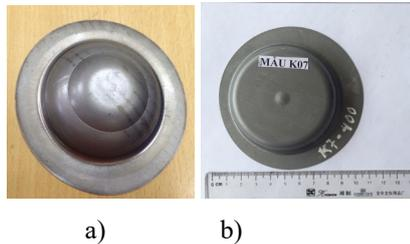
**Fig. 16.** (a) two-step product; (b) one-step product (after the height of the second step is reduced to zero)
