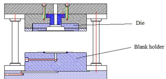
Fig. 7. Experimented die drawing
