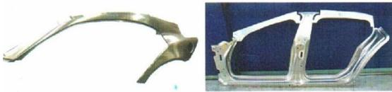
Fig. 1. Some hydrostatic-formed parts [1]
