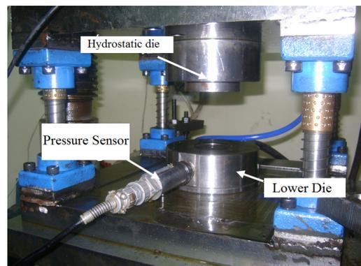
**Fig. 10.** Overall single sheet metal hydrostatic die
