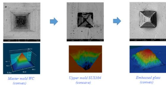
Fig. 3. Fabrication principle of microstructured mold
