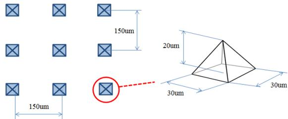
Fig. 4. Size of pyramid array
