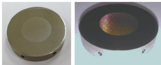
Fig. 5. Microstructured-upper mold before (left) and after (right) coated
