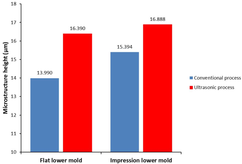
Fig. 10. Pyramid height after experiments
