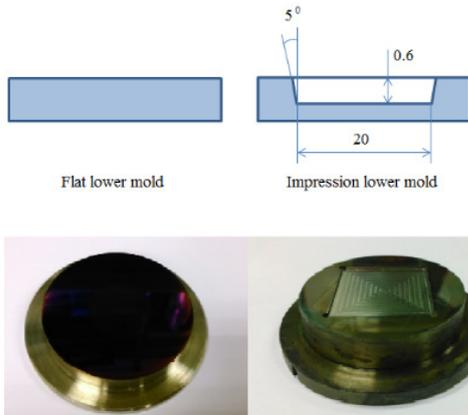
**Fig. 6.** Flat (left) and impression (right) lower molds
