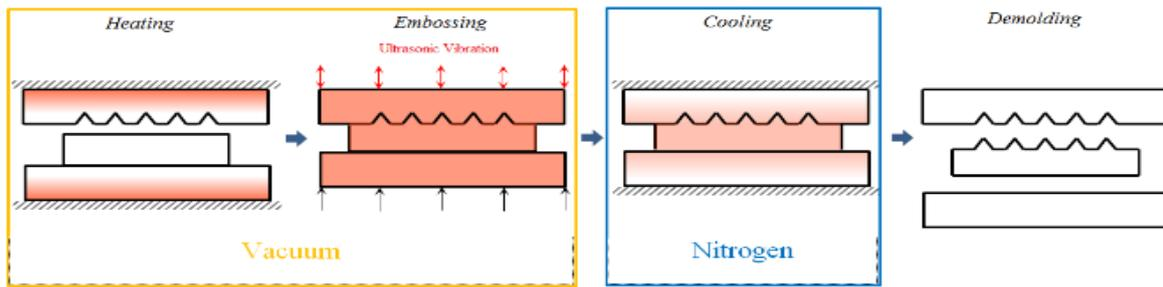
Fig. 1. Stages of ultrasonic vibration-assisted hot glass embossing process
