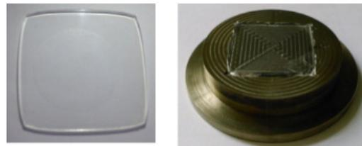
**Fig. 8.** Embossed glass using flat (left) and impression (right) lower molds
