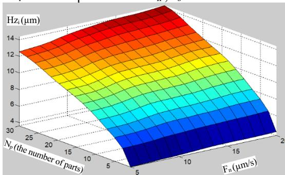
Fig. 9. The relationship between the amount of wear  $H_z_i$  and the input variables  $F_n, N_p$
