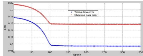
**Fig. 5.** Error value graph according to the number of iterations during the ANFIS training process
