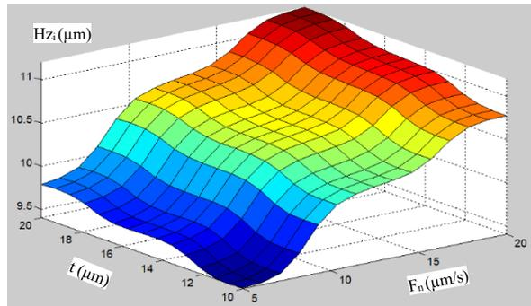
Fig. 8. The relationship between the amount of wear  $H_z_i$  and the input variables  $F_n, t$
