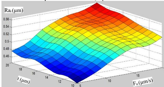
Fig. 11. The relationship between the surface roughness of part  $Ra_i$  and the input variables  $F_n, t$
