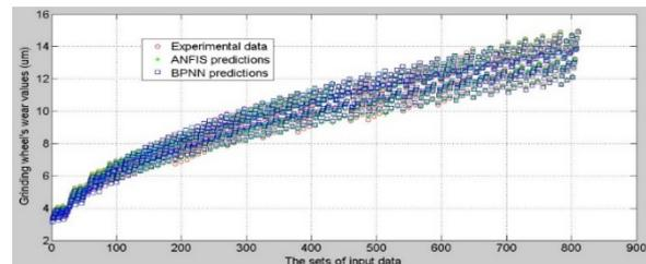
**Fig. 6.** The comparison of ANFIT predictions, BPNN predictions and experimental data values at the different sets of input data
