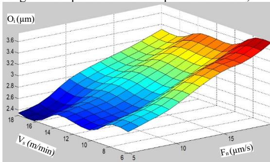
Fig. 13. The relationship between the oval level of part  $O_i$  and the input variables  $F_n, V_s$
