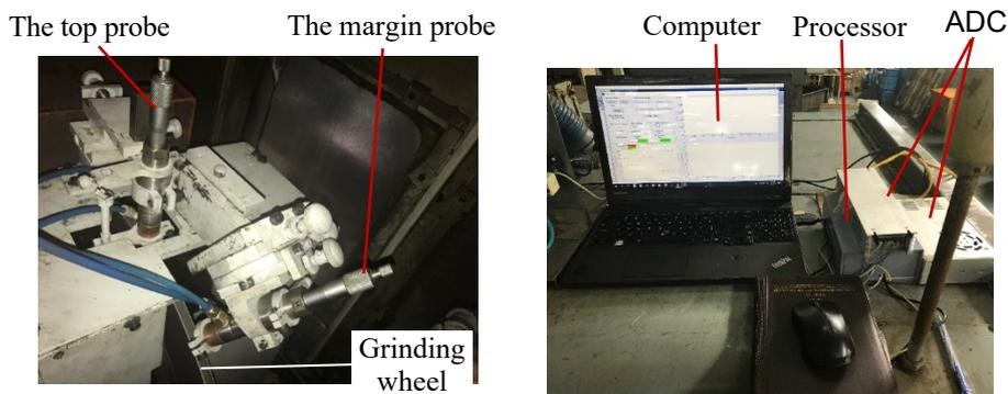
Fig. 3. The model diagram of the experimental system [1-3]
