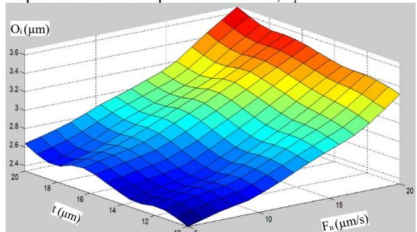
Fig. 14. The relationship between the oval level of part  $O_i$  and the input variables  $F_n, t$
