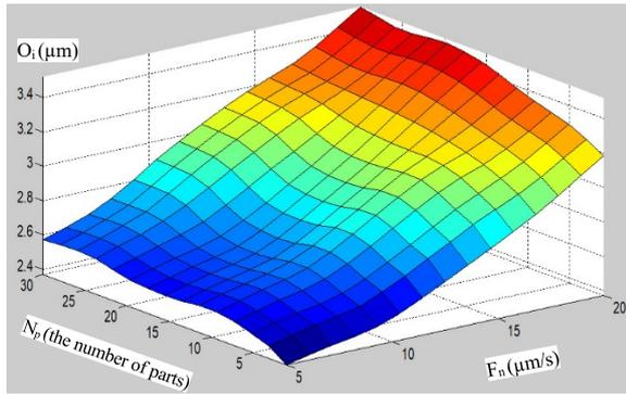
**Fig. 15.** The relationship between the oval level of part  $O_i$  and the input variables  $F_n, N_p$
