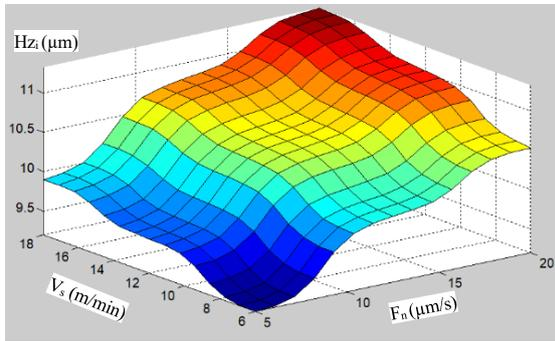
Fig. 7. The relationship between the amount of wear  $H_z_i$  and the input variables  $F_n, V_s$
