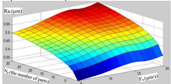
Fig. 12. The relationship between the surface roughness of part  $Ra_i$  and the input variables  $F_n, N_p$
