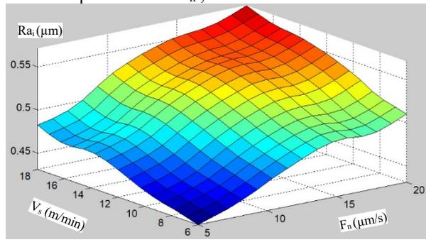
Fig. 10. The relationship between the surface roughness of part  $Ra_i$  and the input variables  $F_n, V_s$
