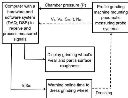
**Fig. 4.** Online-monitoring model of grinding wheel's wear and part's surface roughness for profile grinding ball bearing's inner ring groove [9, 10]
