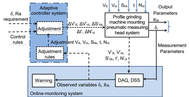
Fig. 3. The functional diagram of system to monitor online grinding wheel's wear and part's surface roughness for profile grinding ball bearing's inner ring groove [9, 10]
