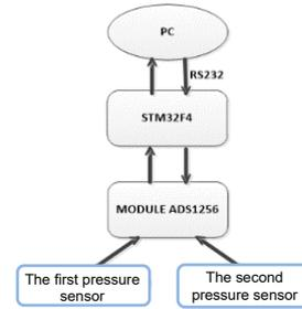
Fig. 6. The diagram of control circuit principle
