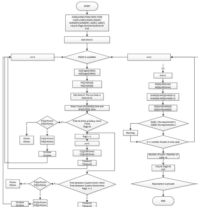
Fig. 8. Algorithm for interface software program to find grinding wheel's wear value
