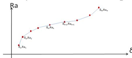
Fig. 7. Construction characteristic line  $R_a(\delta)$  between grinding wheel's wear and part's surface roughness based on experiment
