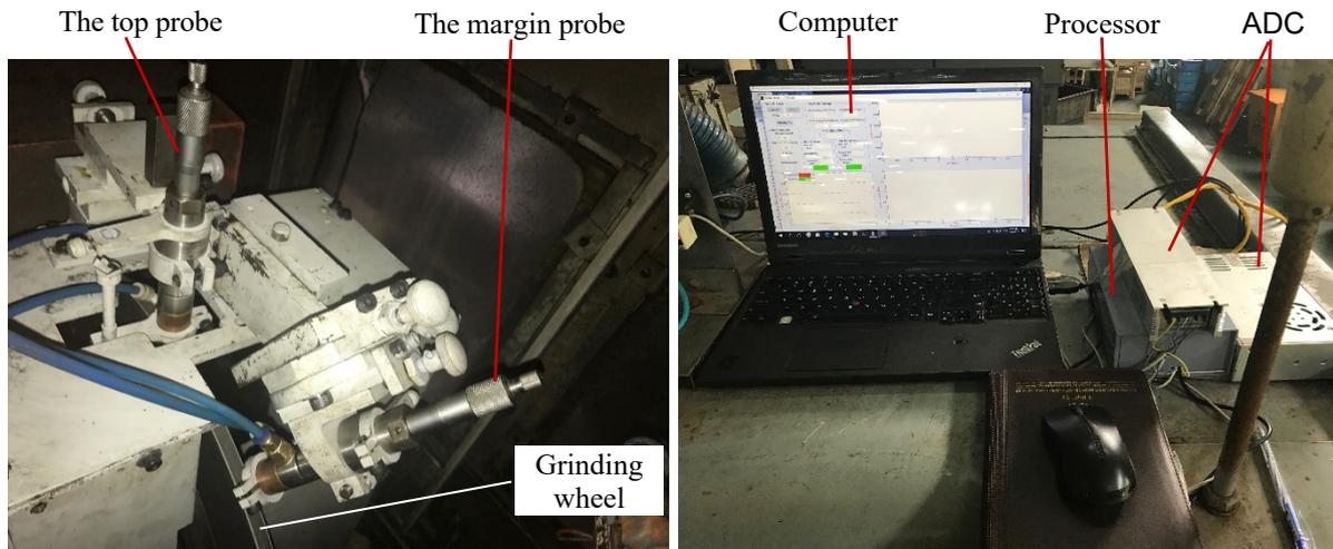
Fig. 9. Experimental system measuring grinding wheel's wear for profile grinding ball bearing's inner ring groove after mounting two probes onto profile grinding machine 3MK136B [2, 3]
