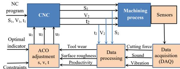
Fig. 2. The general structure of an adaptive control system [9, 10]
