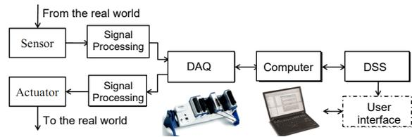
Fig. 1. The structure diagram of an online monitoring system [10]
