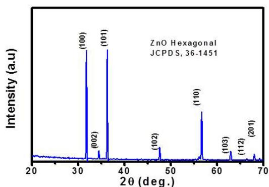
**Fig. 2.** XRD pattern of the single ZnO microbelt.
