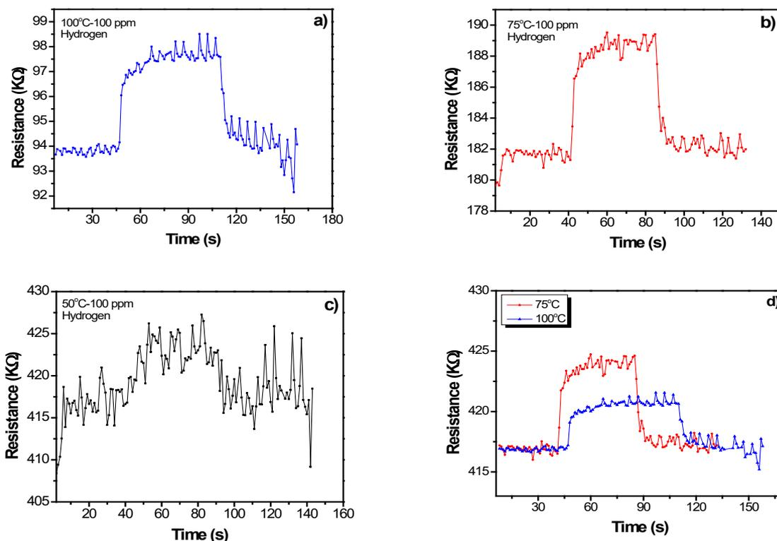
**Fig. 4.** Response transients of the hybrid sensor ZnO microbelt-porphyrin to 100 ppm hydrogen at different working temperatures: a) 100°C, b) 75°C and c) 50°C. d) Response transients of the hybrid sensor to 100ppm of H<sub>2</sub> gas, at different working temperatures (red line: 75°C, blue line: 100°C).
