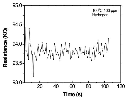
**Fig 3.** Response transients of the ZnO microbelt to 100 ppm of hydrogen at  $100^\circ\text{C}$ .
