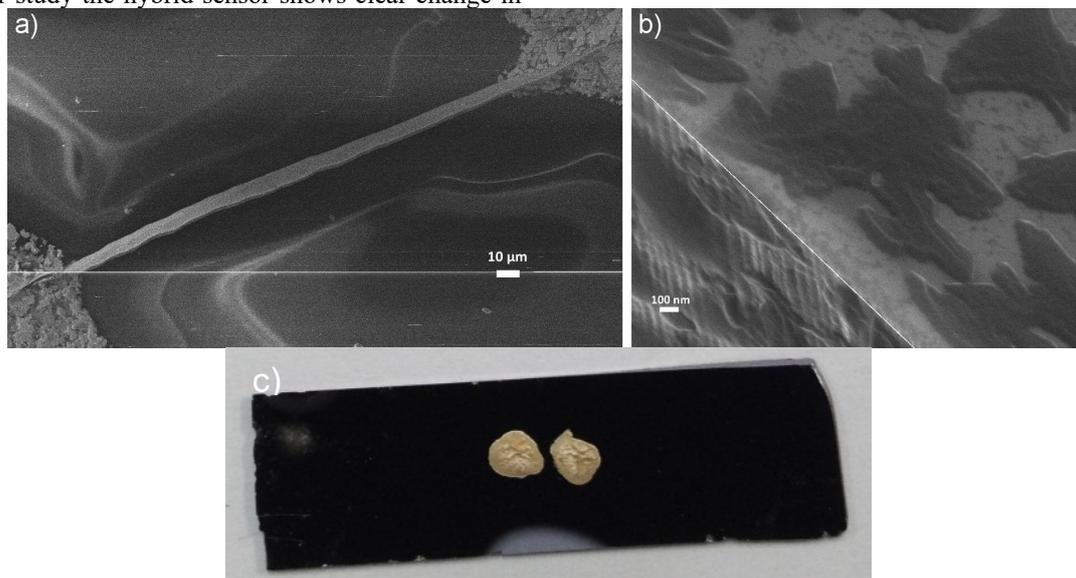
**Fig. 1.** SEM images: a) single ZnO microbelt bridging two silver paste drops and b) functionalized microbelt surface (the dark spots are H<sub>2</sub>TPPF islands on the top surface of the ZnO belt). c): optical image of the whole sensor.
