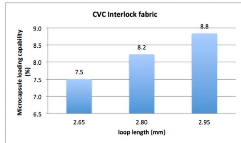
Fig. 3. Influence of loop length on microcapsule loading capability of CVC Interlock fabrics
