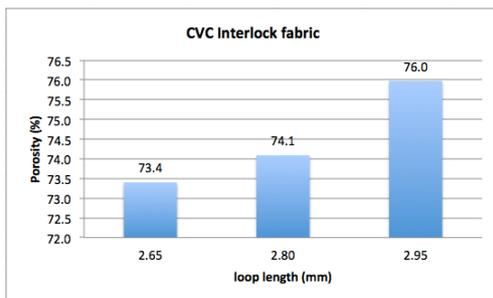
Fig. 8. Influence of loop length on porosity of CVC Interlock fabric
