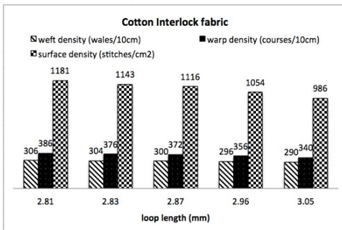
Fig. 4. Influence of loop length on weft density, warp density and surface density of Cotton Interlock fabric
