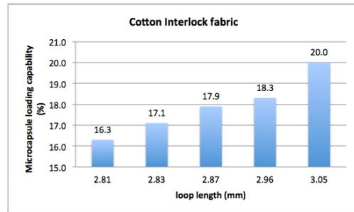
Fig. 2. Influence of loop length on microcapsule loading capability of Cotton Interlock fabrics
