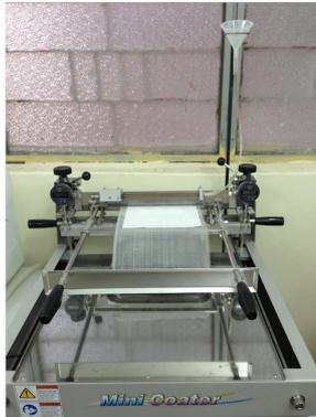
Fig. 1. Experimental coating equipment Mini Coater
