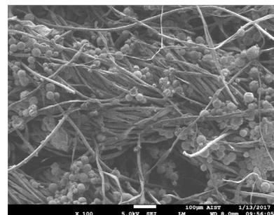
Fig. 6c. Microcapsule-contained CVC fabric with loop length of 2.95 mm
