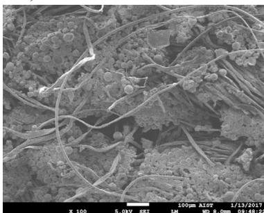
Fig. 6a. Microcapsule-contained CVC fabric with loop length of 2.65 mm
