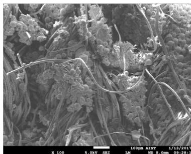
Fig. 6b. Microcapsule-contained CVC fabric with loop length of 2.80 mm
