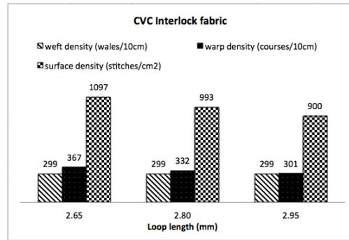
Fig. 5. Influence of loop length on weft density, warp density and surface density of CVC Interlock fabric
