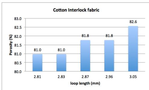
Fig. 7. Influence of loop length on porosity of Cotton Interlock fabric
