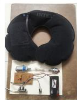
Fig. 8b. Airbag after inflation
