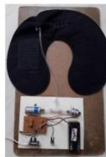
Fig. 8a. Complete kit before inflation
