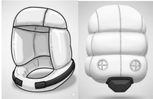
Fig. 9. Illustration of the proposed airbag showing the front and back views
