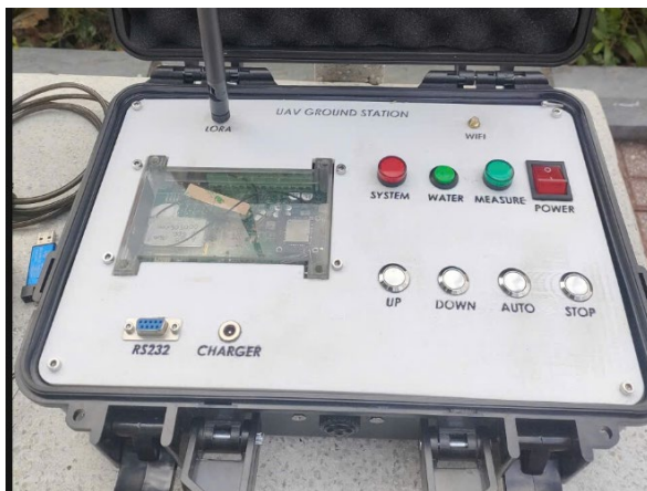
Fig. 5. The ground control station box
