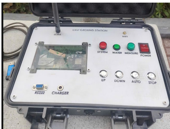
Fig. 5. The ground control station box
