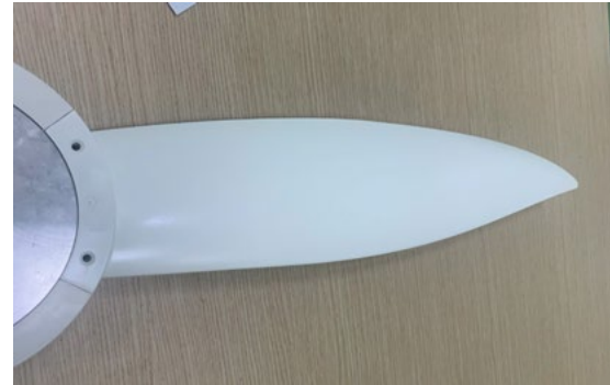
Fig. 27. Air blade prototype (PC anti-shrink material)
