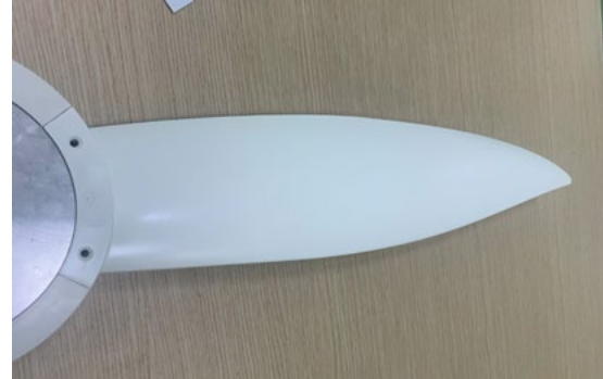
Fig. 27. Air blade prototype (PC anti-shrink material)
