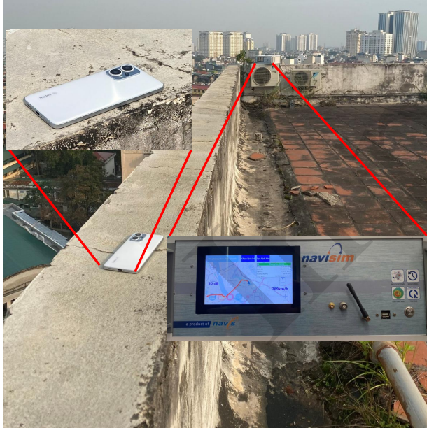
Fig. 6. Setup for the mixed environment with authentic and spoofed signals.
