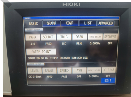
Fig. 4. Impedance analyzer configuration
