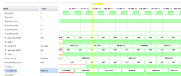
Fig. 5. Post-simulation waveform verifying the functionality of the polynomial vector addition accelerator
