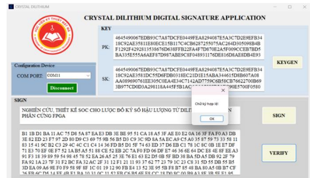
Fig. 7. Graphical interface of the FPGA-based CRYSTALS-Dilithium signature system showing successful key generation and signature verification
