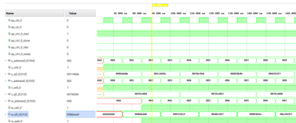
Fig. 5. Post-simulation waveform verifying the functionality of the polynomial vector addition accelerator
