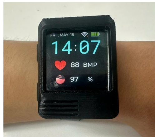
Fig. 10. The physically realized smartwatch prototype for heart rate and SpO 2 monitoring
