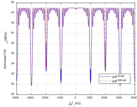
Fig. 2. The theoretical  $C/N_0$  of the satellite PRN01 in the presence of CWI
