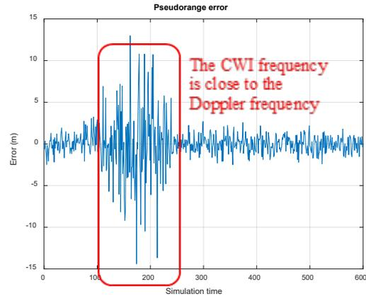
Fig 5. The effect of CWI on GNSS pseudorange error
