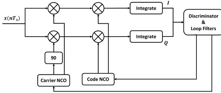
Fig 1. Tracking stage of GNSS Receivers
