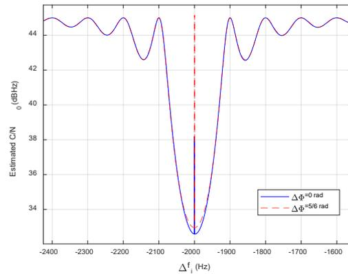
Fig. 3. The theoretical  $C/N_0$  of the satellite PRN01 in the presence of CWI when the frequency offset is -2000 Hz.
