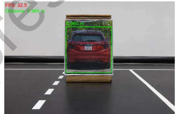
Fig. 7. Frontal-obstacle detection and monocular distance estimation using the camera mounted on the 1:10-scale vehicle
