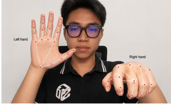
Fig. 4. Hand-posture detection in the driver-monitoring subsystem
