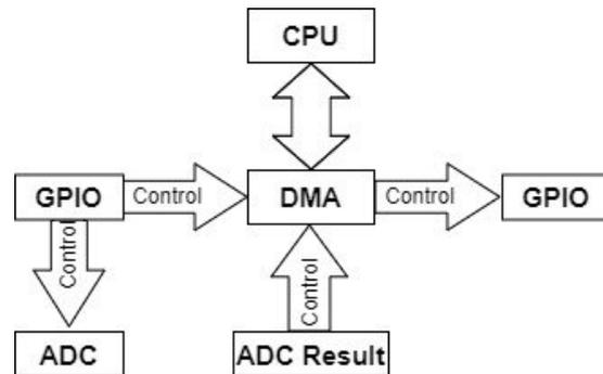
Fig. 8. Block diagram of peripheral operations
