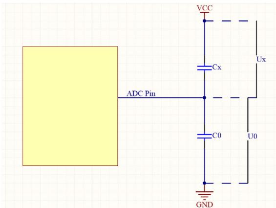
Fig. 2. Principle of voltage measurement of microprocessor
