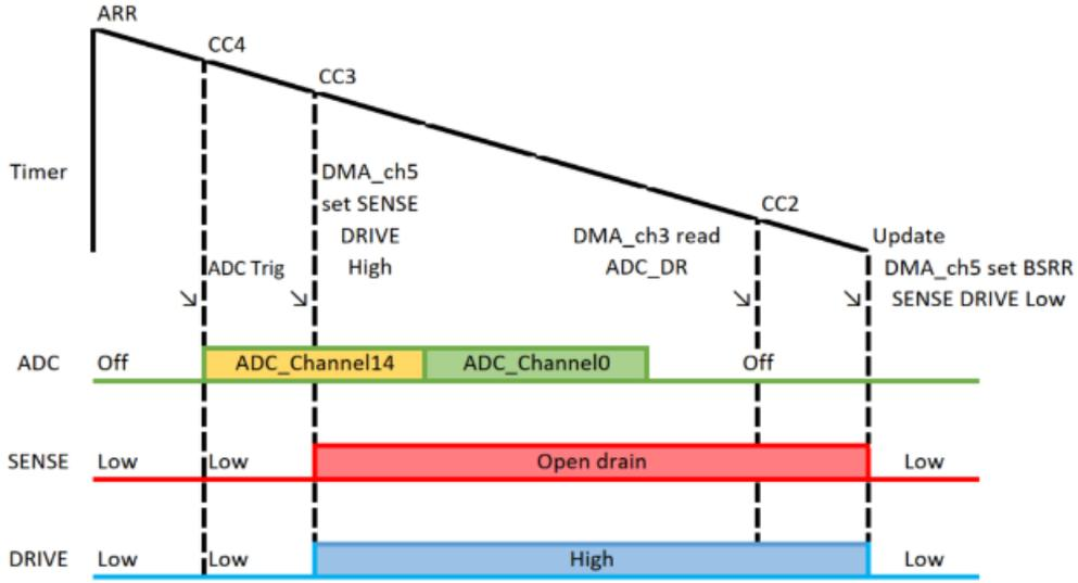
Fig. 9. Timeline of measurements
