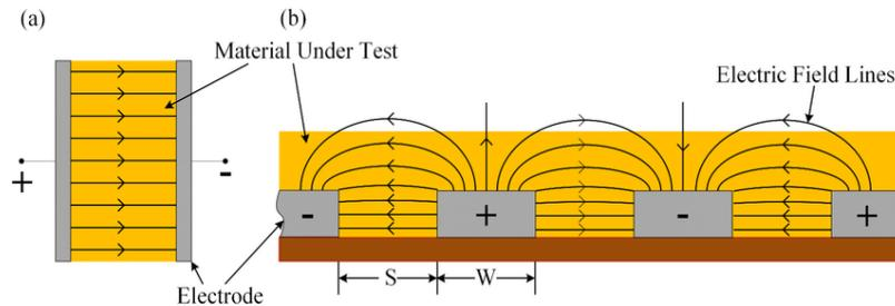
Fig. 1. Electromagnetic field of the capacitor: a) parallel plate capacitor b) coplanar plate capacitor
