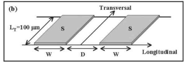
Fig. 11. Parameters of the pole plate
