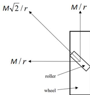
Fig. 1 Forces acting at the ground contact point of the Mecanum wheel's roller
