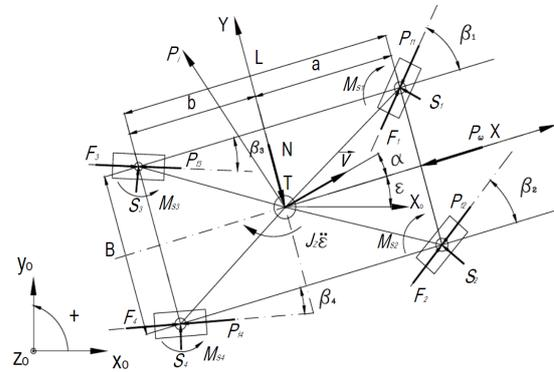
Fig. 5. Forces and moments acting on a running vehicle
