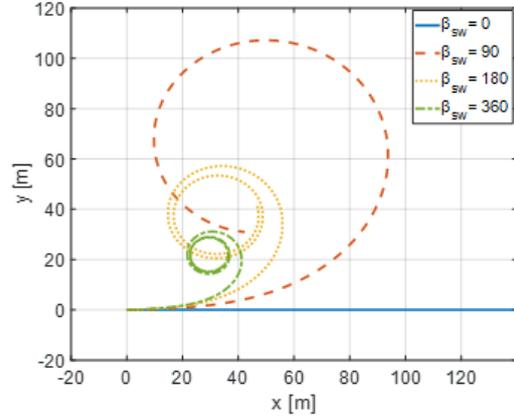
Fig. 12. Motion trajectories of free running vehicle with the steering wheel turned
