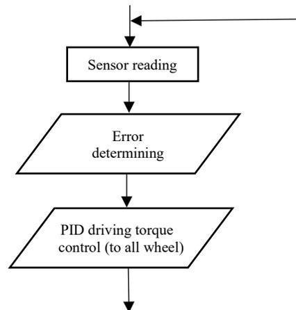
Fig. 16. Main loop of motion direction control algorithm by regulating the driving torque to the wheels
