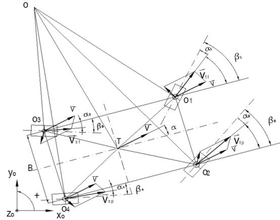
Fig. 7. Side deflection angle of tire
