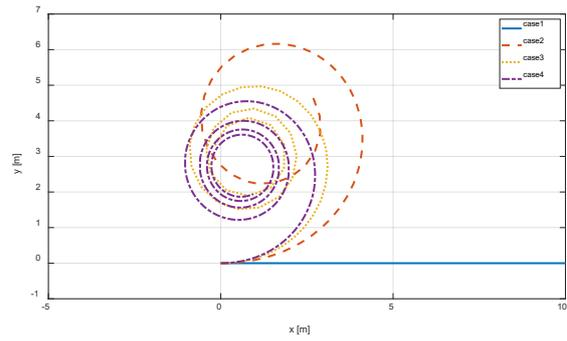
Fig. 4. Motion trajectory of the vehicle using the Mecanum wheels when moving in curved line
