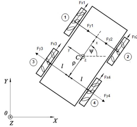
Fig. 2 Force and torque acting on the AGV using Mecanum wheel
