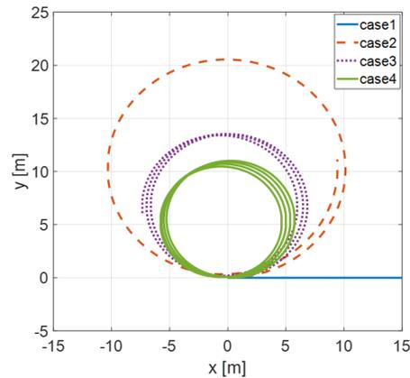
Fig. 10. The motion trajectory of vehicle with different values of driving torque supplied to the left and the right wheels
