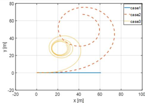
Fig. 14. The motion trajectory of vehicle with different values of driving torque supplied to the left and the right wheels (without turning of the steering wheel)
