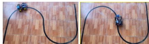
Fig. 17. Positions of vehicle prototype moving along the guiding line by regulating the driving torque to the wheels
