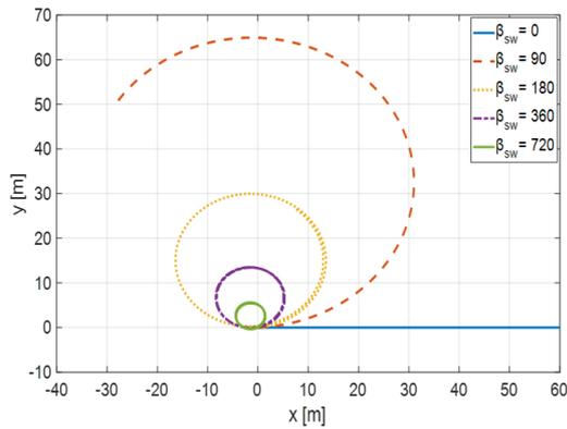
Fig. 8. The vehicle's motion trajectories with constant values of turned angle of steering wheel
