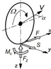
Fig. 6. Forces and torques at the contact point of the wheel with the road surface
