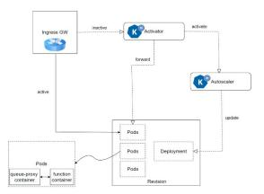
Fig. 6. Key components involved in implementing the auto-scaling or rollback of Knative
