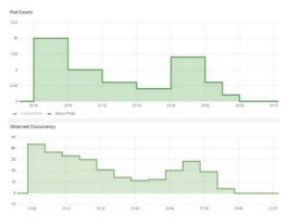
Fig. 13. Knative's process of automatically changing the number of Pods running functions according to the input traffic load
