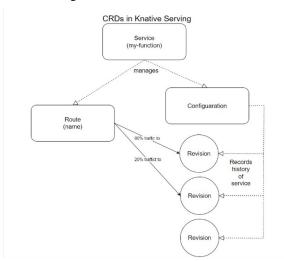
Fig. 4. Block diagram of components in Knative Serving
