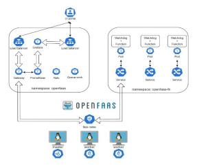
Fig. 10. Deployment diagram of system components of OpenFaaS platform
