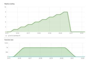
Fig. 12. OpenFaaS's process of automatically changing the number of Pods running functions according to the input traffic load
