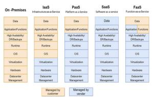
Fig. 1. Comparison of cloud computing service delivery models
