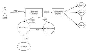
Fig. 5. Operational flow during OpenFaaS auto-scaling or rollback
