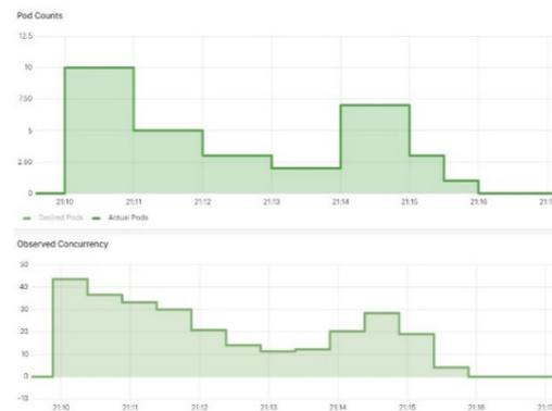
Fig. 13. Knative's process of automatically changing the number of Pods running functions according to the input traffic load
